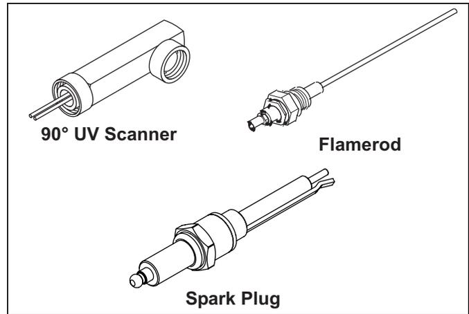
Figure 3.3. Flame Sensor Components
