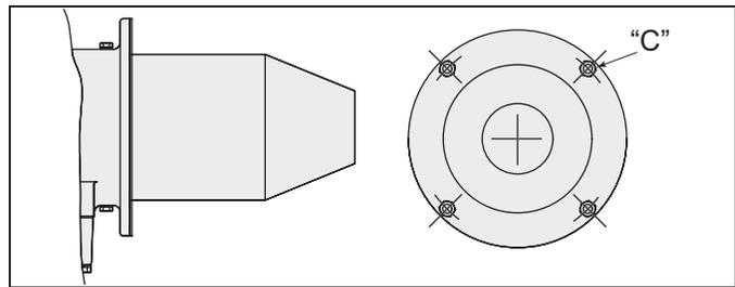
Figure 3.4. Burner Attachment
